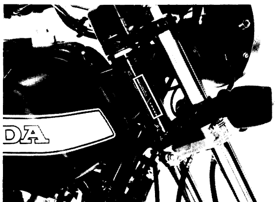
The frame serial number is stamped on the steering head right side.
